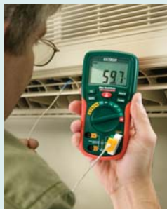
Type K Temperature function (EX230 model)
