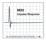
no capacitors in the signal path providing excellent phase response. This also allows the microphone(s) to feed long signal lines up to 300 feet (91m) and maintain the full frequency response of the microphone at the other end of the line, without any loss in high frequencies.
