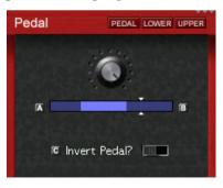
The minimum and maximum value can be set with the knobs A and B. The arrows show the actual position of the pedal. The pedal function can be inverted with knob C.
