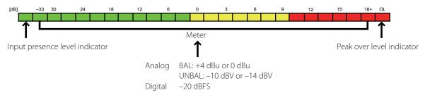
The meter scale has 26 dot LED consisting of a 24 dot level meter, an input presence level indicator and a peak over level indicator. You can choose from four combinations of PEAK and VU to be displayed on the meter ("DIP switch settings" (□) page 4)).
