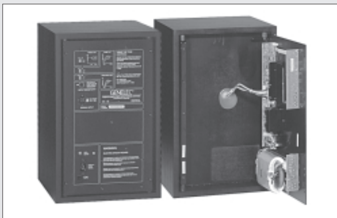
Two channel amplifier is housed in the speaker cabinet
