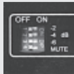
Calibrated 'Tilt' switch. MUTE disconnects the channel for testing.
