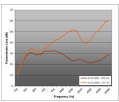
OL 12-0202 – Reference wall before application of Green Glue Noiseproofing Sealant – STC 24
