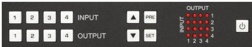
Figure 17 – Control buttons on the front panel
