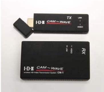
Reliable, compact and affordable, the CW-1 transmits uncompressed full HD 1920x1080. The HDMI type transmitter and receiver system delivers crystal clear images between 30-328ft. With latency less than 1ms, the CW-1 is ideal for real-time wireless monitoring applications. The compact design enables the CW-1 to easily mount on
