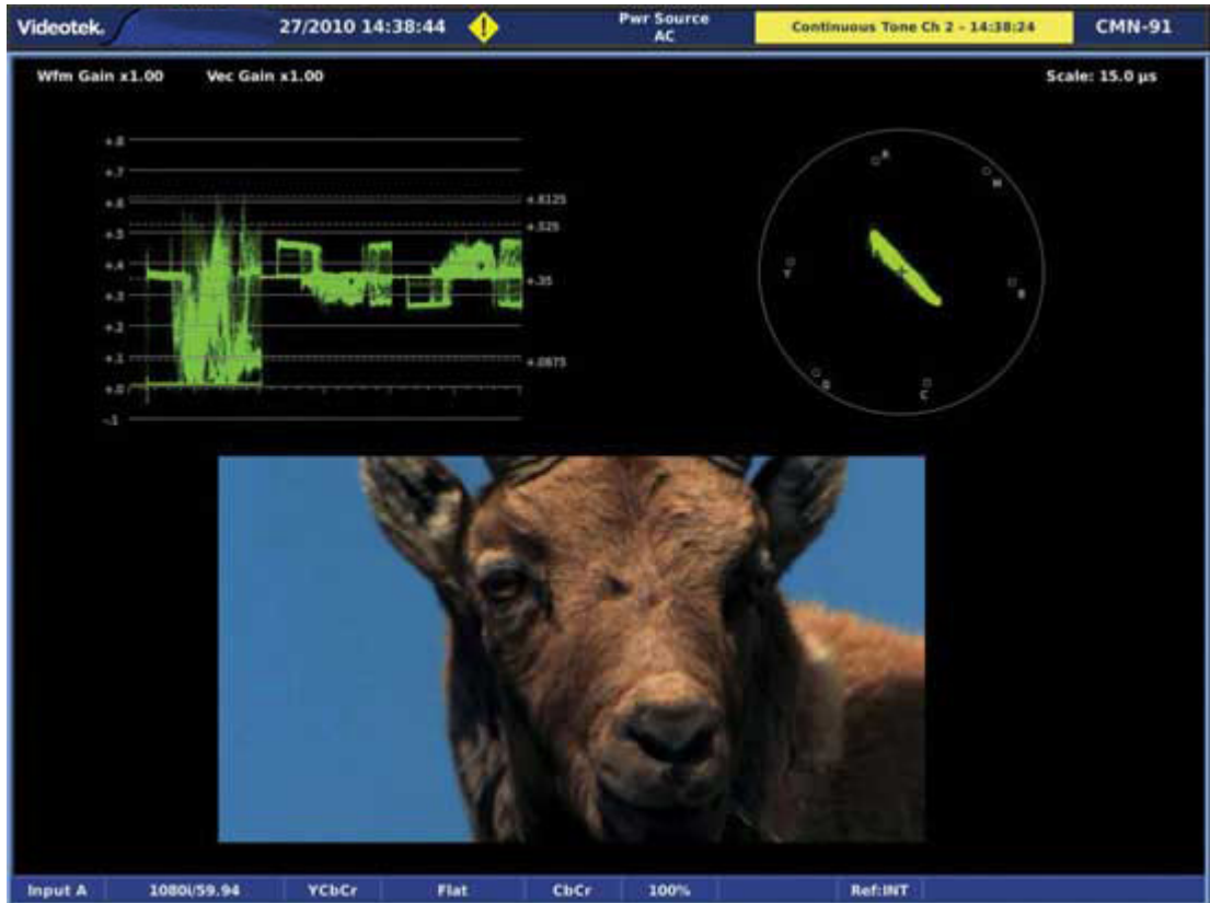
Compact Monitor Series screen capture in Overlay mode with waveform, vector and PiP display. Each component of the display is individually resizable
