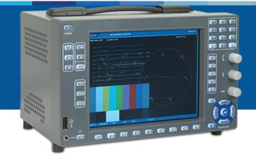
The CMN-91-3GB multiformat signal analyzer with integral LCD is the smallest solution on the market for efficient video and audio signal monitoring. The CMN-91-3GB tests signal quality across all DTV formats up to 3 Gb/s. It possesses two triple-rate SDI inputs and provides selectable waveform, vector, gamut, timing and picture full-screen display.
