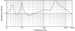
Measurements obtained in full passive crossover mode with no signal processing. Graphs are from unaltered measured data.
