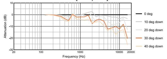
Measurements obtained in full passive crossover mode with no signal processing. Graphs are from unaltered measured data.
