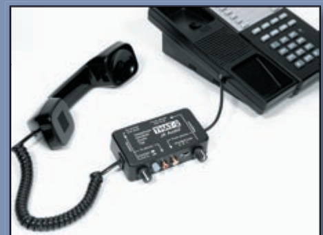
Simply plug THAT-2 between the handset and the base of your phone
