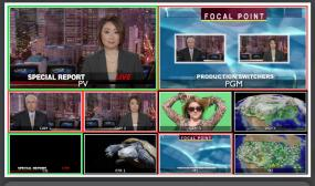
Any input can be routed to any window. PVW / PGM can be displayed in large or small windows with labels. Red (on air) or Green (preview) tally indication.
