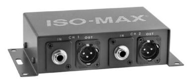
The Iso•Max DB-2PX is a stereo direct box designed to drive unbalanced instrument signals distances to 100 meters (300') or more without high frequency loss or introducing noise into the signal path.
