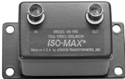
The Iso•Max VB-1BB is a single-channel 75 Ω video isolator for composite (baseband) video that is used to eliminate 60 cycle 'hum bars' even where ground voltage differences are very large such as in surveillance video systems, night clubs, video walls, broadcast stations, and industrial plants.
