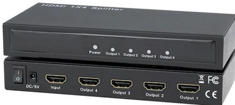
The KanexPro 1x4 HDMI Mini Distribution Amplifier is a compact, lightweight HDMI splitter that distributes one HDMI input into four identical outputs. The conforming outputs also have the ability of buffering and amplifying all the HDMI signals. It can achieve long distance transmission of HDMI signals up to 50 feet (15 meters). It is compatible with computer resolutions up to WUXGA (1920x1200 @ 60Hz), including HDTV 1080p/60.
