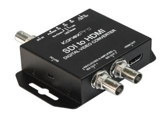
The KanexPro next generation of SDI to HDMI converters are designed for connecting your professional SDI video equipment to any HDMI display or consumer based TV's. It accepts SD, HD or 3G-SDI signals and converts it to HDMI maintaining signal integrity of the original image and resolution. The converter also has two SDI loop outputs for sending re-clocked SDI signals and connecting to down-stream equipment.
