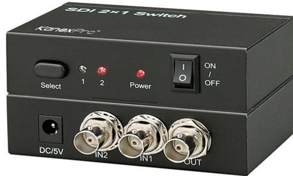
The KanexPro SDI switcher is a 2 input, one output switcher designed to switch two SDI sources to one SDI monitor or display. For optimum performance the SDI switcher is loaded with re-clocking technology to drive the signal at longer distances and supports SDI, HD-SDI and 3G-SDI signals.
