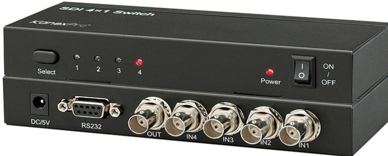
The KanexPro SDI switcher is a 4 input, one output switcher designed to switch four SDI, HD-SDI or 3G-SDI sources to one SDI monitor or display output. For optimum performance the SDI switcher can be controlled using RS-232 to switch the inputs. The 4X1 switcher includes re-clocking technology which drives the signal at longer distances and supports SDI, HD-SDI and 3G-SDI signals. It supports multi-stage cascading for adding more SDI components and switchers.
