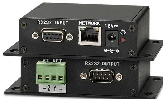
The KanexPro TCPRS2 is a programmable Ethernet control processor designed to integrate IP (internet protocol) with any Matrix Switcher, signal processor, scaler or lighting products. It converts TCP/IP signals to RS-232 or serial commands for devices that needs full control in terms of remote switching, troubleshooting or active monitoring.
