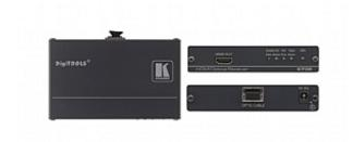
The 670R is a high-performance fiber optic receiver for HDMI signals. The unit receives an optical signal from the 670T and converts the light pulses back to an HDMI signal.
