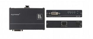
The 671R is a high-performance fiber optic receiver for DVI signals. The unit receives an optical signal that is transmitted over one single fiber optic cable from the 671T and converts it back to a DVI signal.
