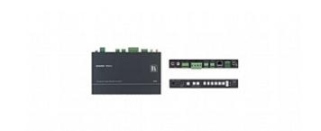
The 906 is a high-performance controllable power amplifier for line-level stereo audio signals. It accepts either an unbalanced stereo audio signal on RCA connectors or a balanced stereo audio signal on a terminal block connector. It delivers a speaker output of 6.8 watts RMS per channel into a  $4\Omega$  load.
