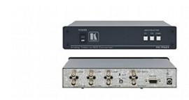
The FC-7501 is a format converter for composite video, s-Video or component video (YUV) signals. It converts either PAL, SECAM, and NTSC composite video, s-Video, or component (YUV) signals into two SDI (SMPTE 259) signals simultaneously.
