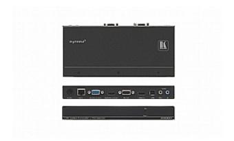
The Kramer KDS-EN3 is an H.264 encoder for HDMI signals up to 1080p60. The KDS-EN3 provides unicast (one-to-one) or multicast (one-to-many) streaming to the KDS-DEC3 decoder or computers running VLC© software. KDS-EN3 can also record content to a network drive for later access.
