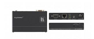
The TP-123EDID is a high-performance twisted pair transmitter for computer graphics video, unbalanced stereo analog audio and unidirectional RS-232 control command signals. It converts the input signals to a twisted pair signal and transmits it over CAT 5 cable to a compatible receiver.
