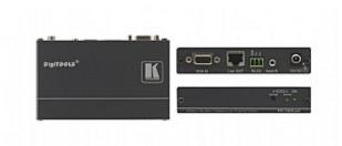
The TP-125-od is a high-performance twisted pair transmitter for computer graphics video, unbalanced stereo audio and bidirectional RS-232 control command signals. It converts the input signals to a twisted pair signal and transmits them over CAT 5 cable to a TP-126-od receiver.
