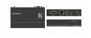
The TP-125xl is an extended range twisted pair transmitter for computer graphics video, unbalanced stereo audio and bidirectional RS-232 control command signals. It converts the input signals to a twisted pair signal and transmits them over CAT 5 cable to a compatible receiver.
