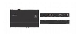
The TP-576 is a DGKat™ twisted pair line driver for HDMI, bidirectional RS-232 and infrared signals. The unit receives an HDMI signal either from a local HDMI source or from a compatible twisted pair transmitter. It decodes the selected signals to the local HDMI, RS-232 and IR outputs and simultaneously transmits them to a compatible twisted pair receiver.
