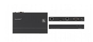
The TP-581T is a high-quality HDBaseT twisted pair transmitter for HDMI, Ethernet 100BaseT, bidirectional RS-232 and IR signals. The TP-581T takes the HDMI, Ethernet 100BaseT, RS-232 and IR input signals and converts them to an HDBaseT twisted pair signal. The TP-582R converts the HDBaseT twisted pair signal back to Ethernet 100BaseT, RS-232, IR and two HDMI outputs, and de-embeds the audio to S/PDIF and TOSLINK® audio outputs.
