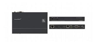
The TP-582T is a high-quality twisted pair transmitter for HDMI, Ethernet 100BaseT, bidirectional RS-232 and IR signals. The TP-582T selects one of two HDMI inputs, and converts it with the Ethernet 100BaseT, RS-232 and IR input signals to an HDBaseT twisted pair signal. The TP-582R converts the HDBaseT twisted pair signal back to Ethernet 100BaseT, RS-232, IR and two HDMI outputs, and de-embeds the audio to S/PDIF and TOSLINK® audio outputs.
