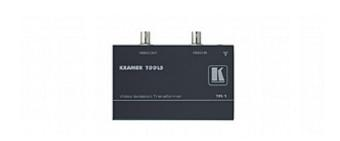
The TR-1 is a high-resolution isolation transformer for composite video signals. It completely isolates devices to eliminate video hum, ground loops, and DC offsets that can degrade picture quality.
