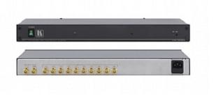
The VM-10HDxI is a high-performance distribution amplifier for 3G HD-SDI signals. The unit takes one input, provides reclocking and equalization and distributes the signal to ten identical outputs.
