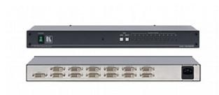
The VM-12HDCP is an HDCP-compliant distribution amplifier for DVI-D signals with resolution up to 1080p or UXGA. It reclocks and equalizes the signal and distributes it to twelve identical outputs.
