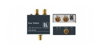
The VM-2HD is a high-performance distribution amplifier for HD-SDI signals. It takes one input, provides reclocking and equalization and distributes the signal to two identical outputs.
