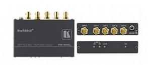
The VM-4HDxl is a high-performance distribution amplifier for 3G HD-SDI signals. The unit takes one input, provides reclocking and equalization and distributes the signal to four identical outputs.
