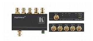
The VM-5HDxIn is a high-performance distribution amplifier for 3G HD-SDI signals. The unit takes one input, provides reclocking and equalization, and distributes the signal to five identical outputs.
