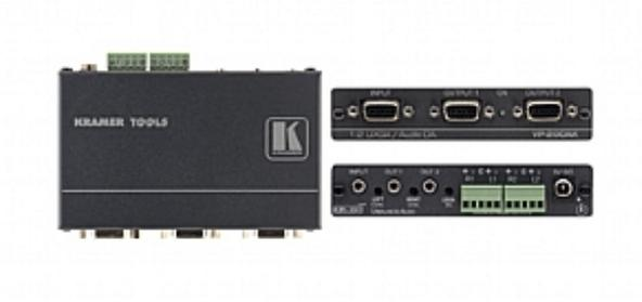
The **VP-200AK** is a high-performance distribution amplifier for computer graphics video signals, with resolutions up to and exceeding UXGA, and unbalanced stereo audio. It takes a computer graphics video and stereo audio input and outputs two computer graphics video, two balanced, and two unbalanced stereo audio signals.
