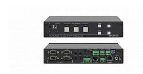
The VP-31KSi is a high-performance analog step-in switcher for computer graphics video with resolutions up to WUXGA and unbalanced stereo audio signals. The unit can switch any one of three inputs to one computer graphics video, one unbalanced and one balanced stereo audio and one twisted pair output. The VP-31KSi works in conjunction with up to three VGA Remote Control Step-in Modules including the SI-1VGA (for TBUS-10), SI-VGAT (under the table) and WSI-1VGA (for standard TBUSes).
