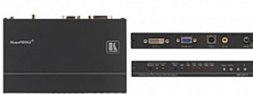
The **VP-417** is a high-performance scaler for composite video and s-Video signals. The unit scales a video signal to a selectable computer graphics video or HDTV output signal on 15-pin HD and DVI-D connectors simultaneously.
