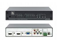
The VP-435 is a high-quality format converter for component video, computer graphics video, HDMI video and unbalanced stereo audio signals. It scales the selected video signal to a computer graphics or HDTV output resolution, embeds the audio and outputs an HDMI signal.
