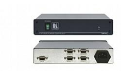
The VP-4xl is a high-performance distribution amplifier for computer graphics video signals with resolutions ranging from VGA through UXGA and higher. The unit takes one input, provides correct buffering and isolation, and distributes the signal to four identical outputs.
