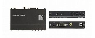
The VP-506 is a high-quality scan converter for down-scaling DVI, computer graphics (VGA) and component video (YPbPr) to PAL or NTSC video. It supports VGA up to UXGA, as well as component resolutions up to 1080p.
