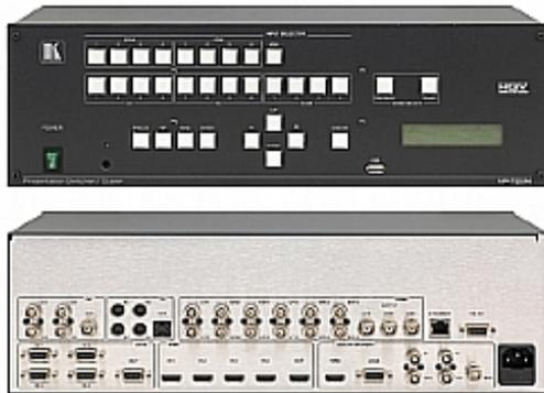
The **VP-725N** is a presentation scaler/switcher with multiple signal format sections. The unit has five independent 4x1 video sections: composite, s-Video (Y/C), component (YUV), computer graphics, and HDMI, plus a single USB input. It also up- or down-scales any video input to a selectable graphics or HDTV output resolution. FTB™ (fade-thru-black) switching technology provides glitch-free switching between sources.
