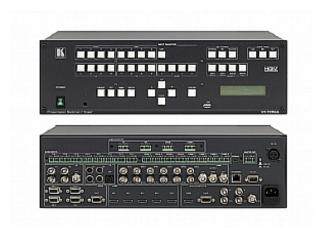
The VP-725NA is a presentation scaler/switcher with multiple signal format sections and balanced stereo audio. The unit has five independent 4x1 video sections: composite, s-Video (Y/C), component (YUV), computer graphics and HDMI, plus a single USB input. It also scales any video input up or down to a selectable graphics or HDTV output resolution and provides glitch-free switching between sources through FTB™ (fade-thru-black) switching technology.
