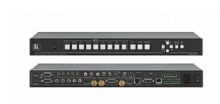
The VP-771 is a high-quality presentation switcher and scaler for a variety of signals. It accepts one of nine inputs: component video, DisplayPort (DP), 3G HD-SDI, two computer graphics, two composite video and two HDMI signals. It scales the video, embeds the audio, and outputs the signal to one HDMI, one computer graphics, one 3G HD-SDI and one DGKat TP, together with digital audio, unbalanced stereo and a 2x10-watt amplified balanced stereo speaker output.
