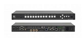
The VP-774AMP is a high-performance presentation switcher and scaler. It accepts one of nine inputs: one DisplayPort (DP), one composite video, two computer graphics, one 3G HD-SDI and four HDMI signals. It scales the video, embeds the audio, and simultaneously outputs the signal to two identical HDMI, one HDBaseT and one 3G HD-SDI output, together with S/PDIF and balanced stereo audio outputs. The unit also includes an audio amplifier and speaker outputs.
