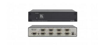
The VP-8K is a high-performance distribution amplifier for computer graphics video signals with resolutions up to and exceeding UXGA. It takes one input, provides correct buffering and isolation, and distributes the signal to eight identical outputs.
