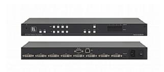
The VS-44HDCP is a high-quality, HDCP compliant 4x4 DVI matrix switcher. It reclocks and equalizes the signals and can route any of the four DVI/HDMI (over DVI-I connectors) inputs to any of the four DVI/HDMI outputs simultaneously.
